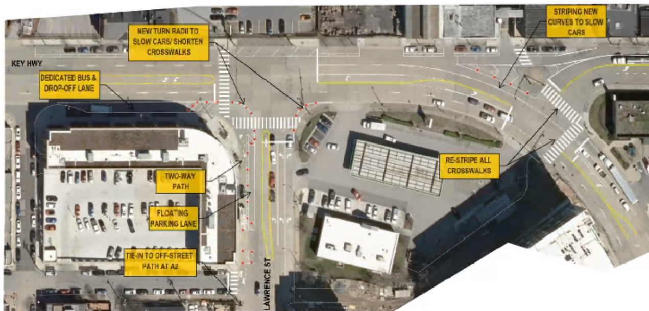
Key Hwy at Lawrence St Restriping & Traffic Calming Quick-Build
